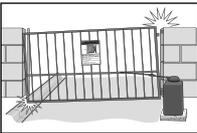
Gate hinges are too tight or broken and the gate is not moving freely. (Swing Only)
