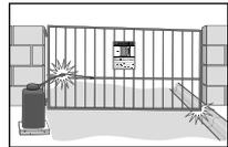
The gate hits the driveway, curb or other, and gets stuck or bent in an awkward position. (Swing Only)
